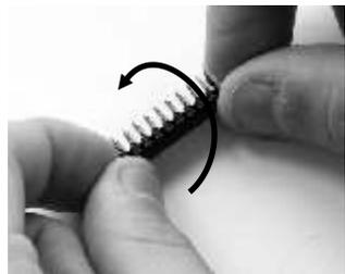
Orient the chips so the label is right side up when the front panel is facing you. Put each chip into its socket and push down firmly. There will be very little space between the chip body and the socket when the chips are plugged in correctly.
