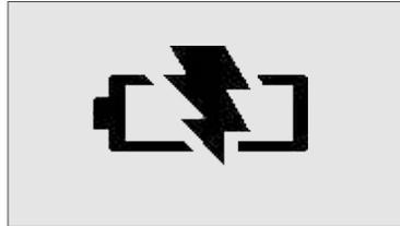
When the charging cable is plugged in and the charger is plugged into the wall outlet, the T2300E displays the charging symbol. The appearance of the charging symbol verifies the charger, cable and throttle are properly connected. After 15 seconds, the throttle shuts off for faster battery charging.
