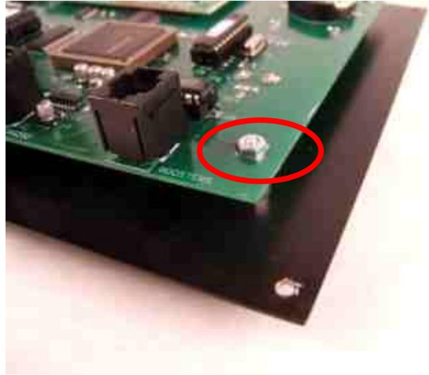
Create a loop of wire, #18AWG or #20AWG. Loosen the nut, place the wire under the nut and then tighten. The other end of the wire goes to your earth ground.
