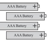
Use four AAA-size batteries. For longest life, use Alkaline-type batteries. The batteries are staggered so the clips don't touch. Squarely snap the batteries into the clip taking care not to bend the somewhat brittle spring clips.
