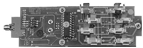
First, unscrew the antenna and set it aside. If your throttle has a shipping screw still attached at the bottom, remove it.
