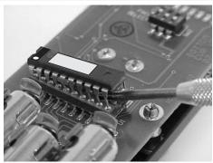
If new features are added to the AirWire throttle, the chip containing the software will have to be changed. Follow the instructions carefully to avoid costly damage to the circuit board. If you would rather have CVP install the chip, please call for authorization. You are responsible for shipping and insurance plus the cost of the chip if any.
