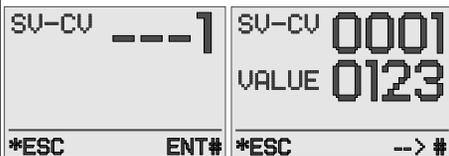
Now key in the value which will be 123 for this example. Finally, push #. The moment the # key is pushed, the decoder will chirp or jump (depends on the decoder) which indicates it has received the command.
