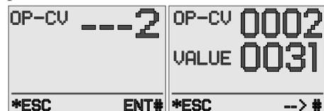
Enter the desired value, 31 for this example. Now push #. The moment the # key is pushed, the new value is sent to the decoder. Some decoders may chirp but not always. If changing a CV related to motion, speed and direction controls remain operational even if in the programming mode. This allows you to try out the new setting.
