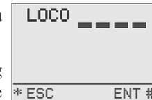
**Step 2:** Key in the numbers of the locomotive decoder. Leading zeroes are not required. For this example, the address is 1234. The display will show each number as it is pressed, with previous numbers moving to the left. If an incorrect number is entered, just continue and enter the proper 4 digits ; no need to start over because **only the last 4 entries** are used when the # key is pushed. You can still cancel by pushing the \* key without any changes.
