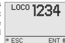
**Step 3:** Push the # key again to tell the throttle to use the address showing on the display. The speed display appears with dashes, followed by 000. Wait until you see the zeroes before changing the speed.
