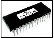
Socketed software chip for easy upgrades
