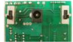
Bottom view of F3 Drop-In showing charger jack and power switches
