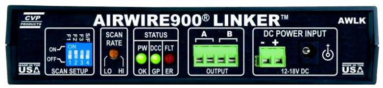
Now it is easier than ever to remotely control your turnouts and other stationary accessories directly from your AirWire throttle. The Linker scans all AirWire frequencies and combines the received activation commands with DC power and sends the combined signal to the companion Activators using a single pair of wires.
