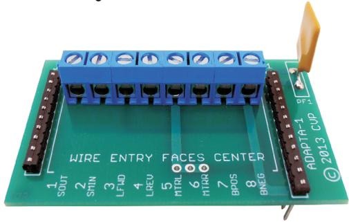
Parts are inserted from the top side and soldering is done on the back or bottom side of the circuit board.
