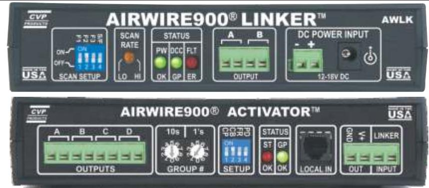
Remote control of turnouts and many types of accessories is easily accomplished with the combination of a single AIRWIRE Linker and one or more AIRWIRE Activators. Together, the Linker and Activator allow your wireless throttle to control items such as switch machines, lights, pumps, relays, solenoids or just about any other type of device found on a typical garden railroad.
